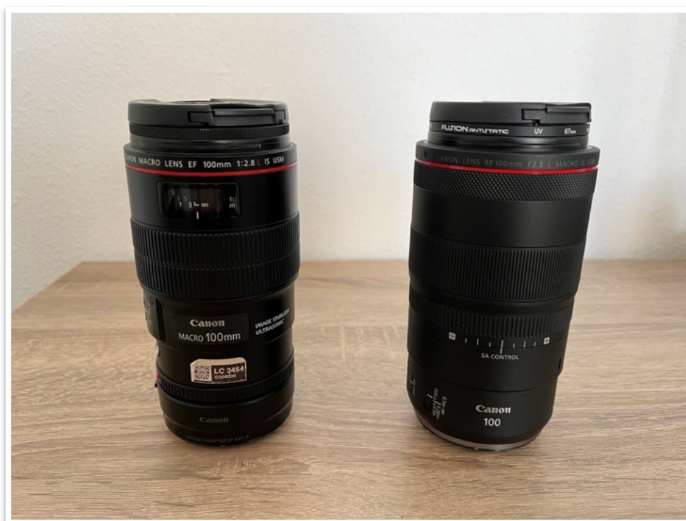
The Canon EF 100 mm on the left, with EF to RF converter, and the RF 100 mm at the right.
