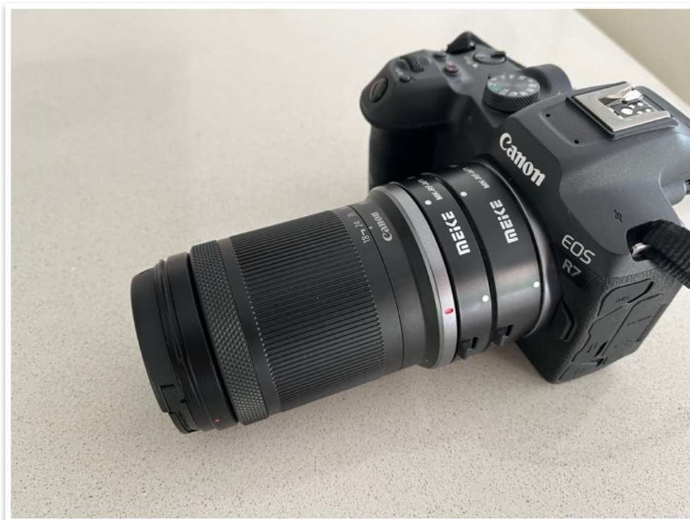
Two extension tubes of 13 mm and 18 mm are placed between the camera and the lens.
